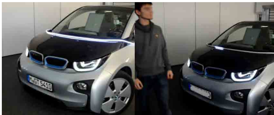
Figure 13: 360° intention-based communication via Light-band: “Pulsing” (left) and “Position-light” (right) (Sorokin et al., 2019)
