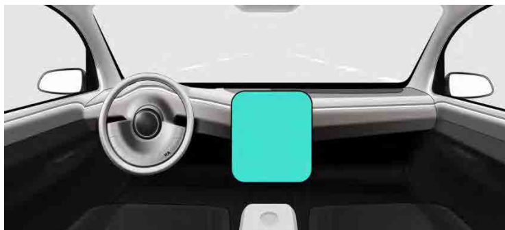
Figure 12: Positioning of the automation display in the interior of the AV
