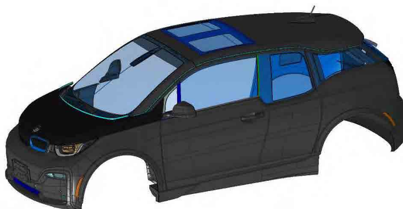
Figure 9: CAD-data of BMW i3s with highlighted eHMI positions for interACT
