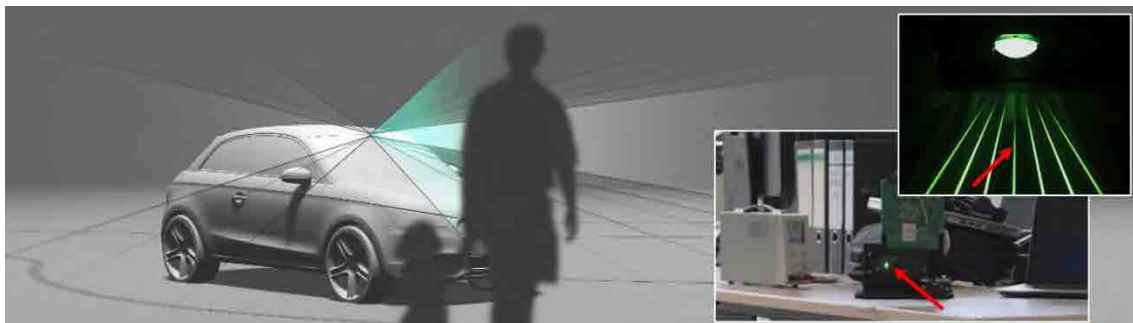
Figure 7: Directed signal lamp idea [Willrodt et al., VDI, 2018].
