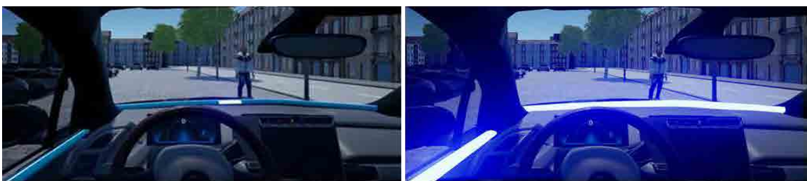
Figure 23: Perception- (left) and intention-based (right) light-band iHMI in the interior of the AV in a parking lot use case
