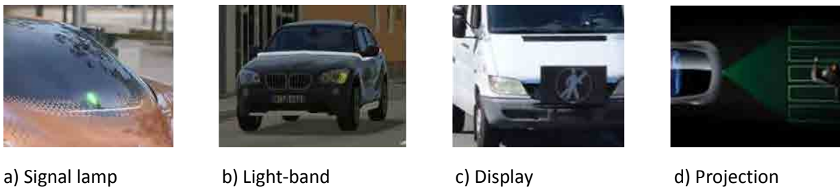
Figure 5: Examples of eHMI technologies (“BMW Vision Next 100,” n.d.; Clamann, Aubert, & Cummings, 2017; Mercedes, 2015; Sorokin & Hofer, 2017)
