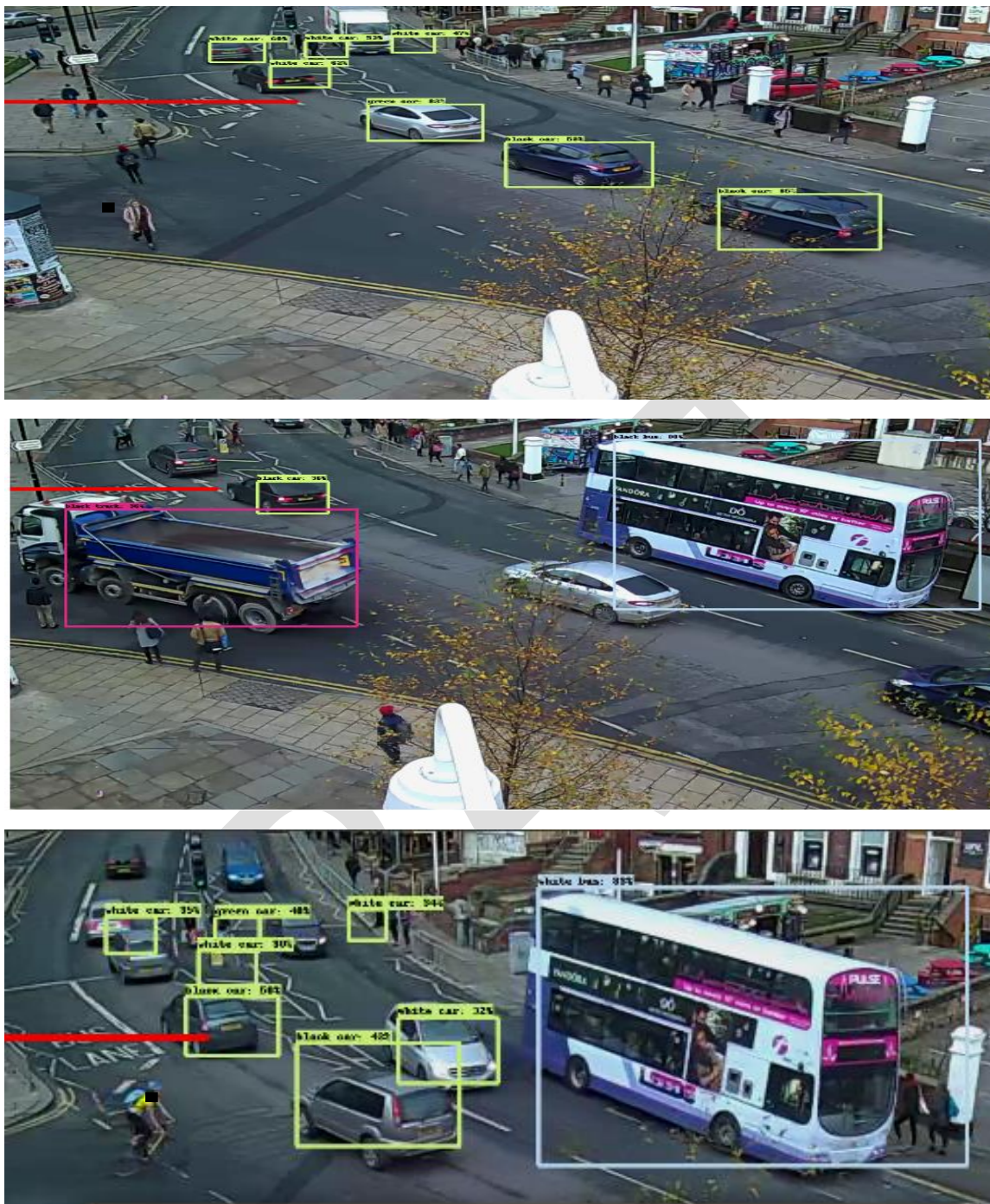
Figure 30: Example images using deep learning detection and classification
