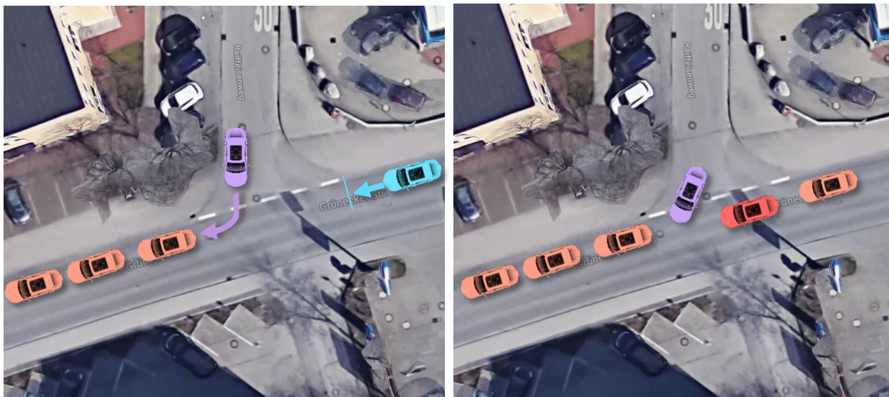
Figure 52: Two different ways one particular use case can play out. Left: vehicle on the priority lane (blue) yields to let the other driver (purple) in, as traffic is congested in front. Right: driver on the side road edges into the intersection, forcing the driver on the priority lane to brake (red).
