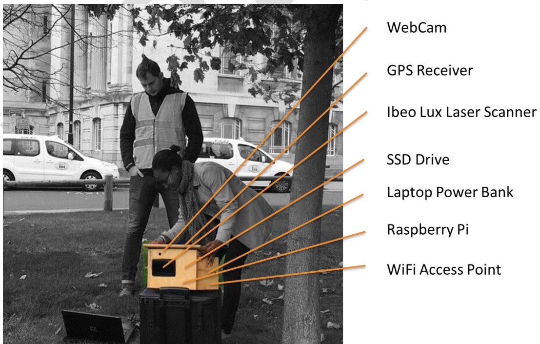
Figure 21: Depiction of the finalized prototype used by Observers in Leeds
