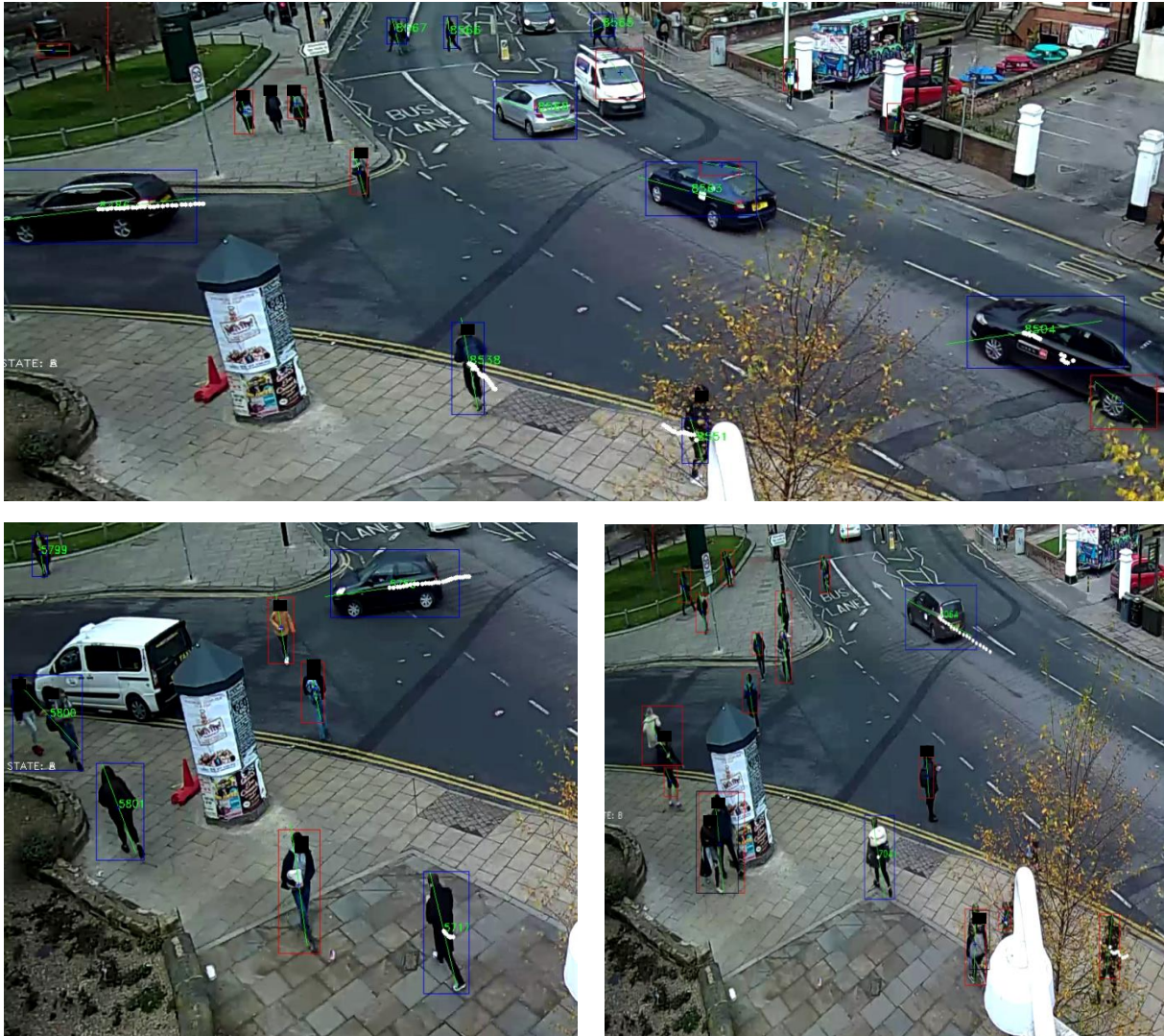
Figure 27: Example images of blob tracking in daytime at the intersection in Leeds
