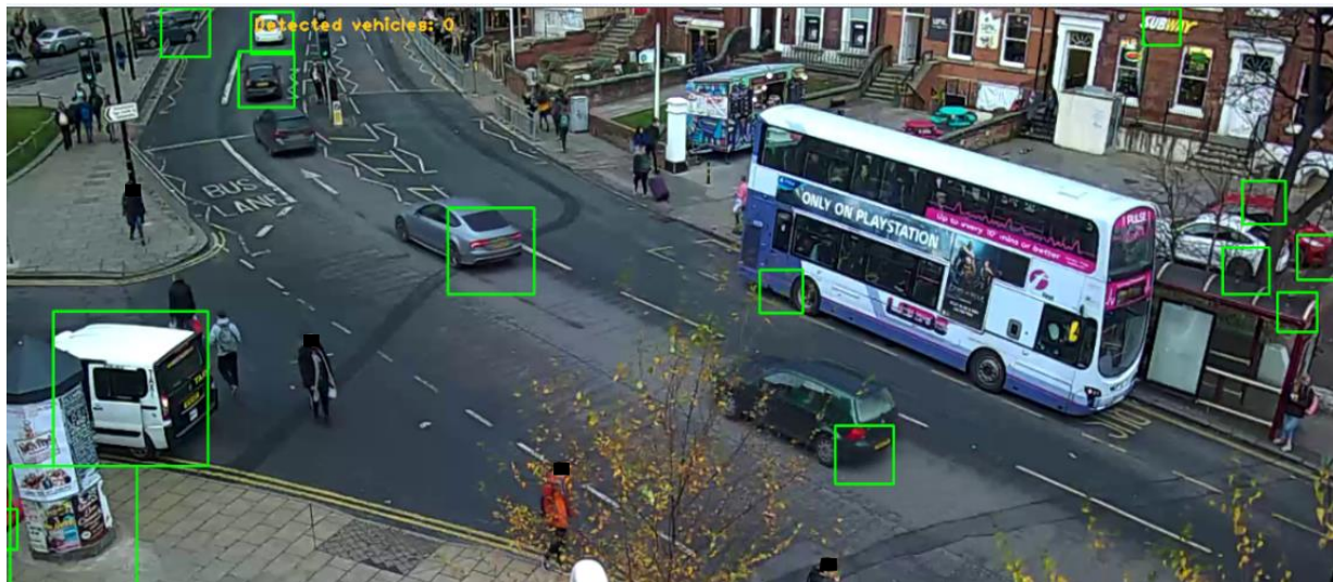
Figure 29: Example image of vehicle detection using HOG + SVM Classifier
