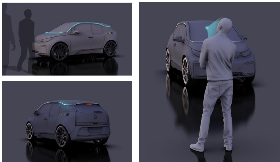
Figure 1: Novel eHMI for interACT AVs – 360° Light Band (left) and Directed Signal Lamp (right).
