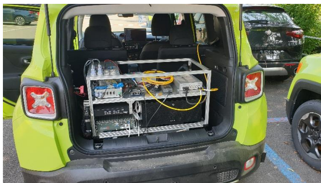
The Cooperation and Communication Planning Unit (CCPU), the brain of the interACT system
