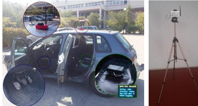
Figure 38: System to log vehicles position, speed and acceleration
