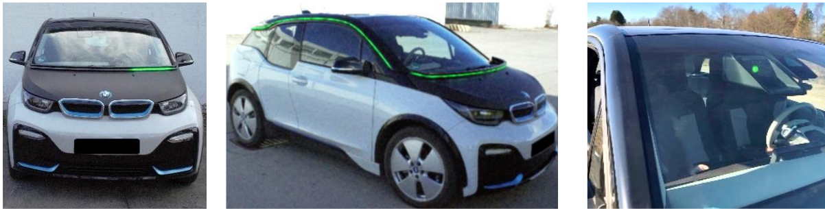
Figure 7: The BMW Wizard of Oz demonstrator with Implemented eHMIs. The LED band displays the perception-based (PB) (l.) and intention-based signalling (IBS and IBF) (c.). The signal lamp (r.) was utilized as a part of the combined signalling (IBS:SL).
