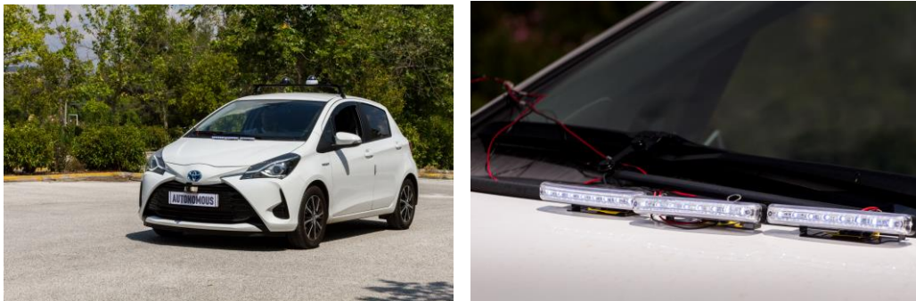
Figure 37: "AV" used in the ICCS study and LED stripe used as external HMI in the condition "AV with eHMI"
