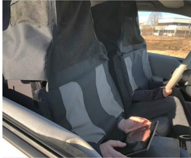
Figure 29: Driver and passenger hidden from the participant's view under seat covers
