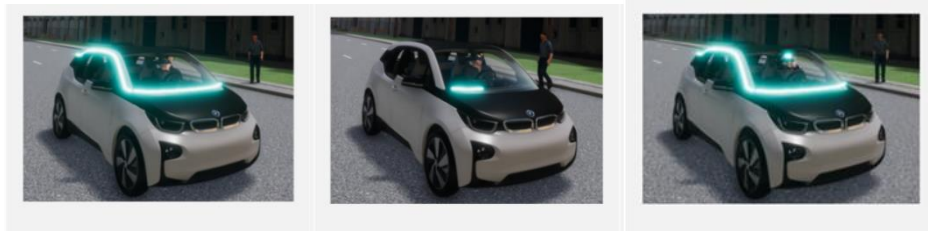
Figure 4: intention-based (left) and perception based light-band (middle) and combined (right) eHMI
