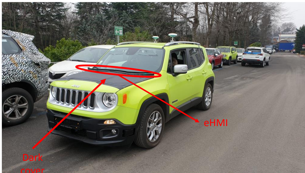
Figure 5: external HMI (eHMI) built by HELLA on the demonstrator vehicle of CRF.
