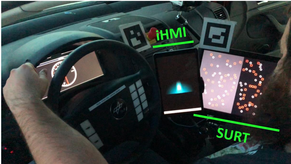
Figure 22: Simulator setup inside the vehicle. The iHMI and SURT were mounted next to the steering wheel on the right.
