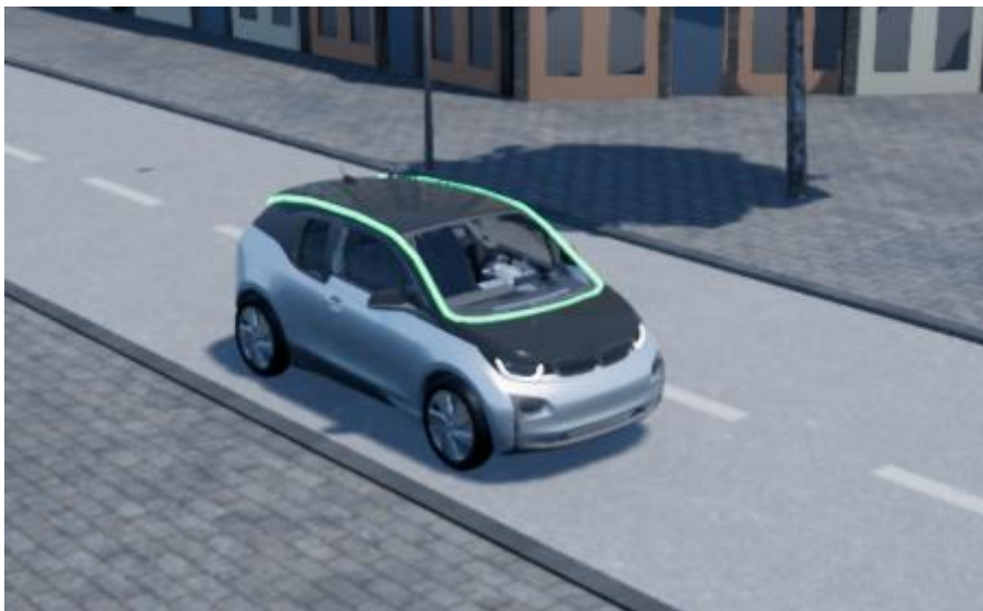
Figure 17: Cyan coloured external HMI on the AV.
