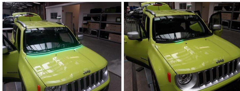
Figure 36: (a) Intention-Based eHMI and (b) Perception-Based eHMI solutions
