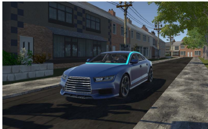
Figure 8: Cyan coloured pulsing light band around the vehicle
