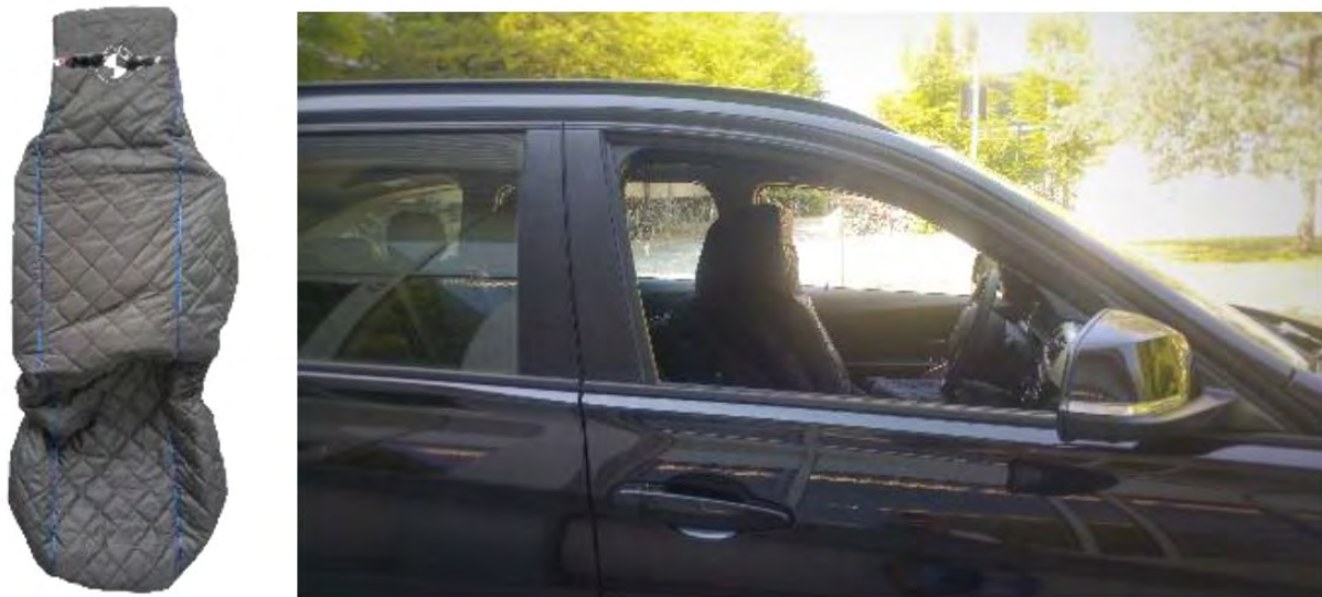
Figure 18: Example of a seat cover to hide the driver and simulate an autonomous driving vehicle (Fuest et al., 2018a)
