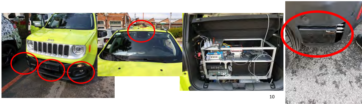
Figure 20: Visualisation of the Perception Platform installed on the CRF vehicle.
