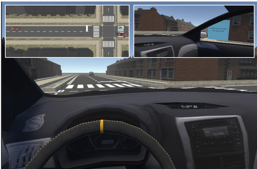
Figure 12: The VR scene in the driver turning scenario. The two insets show a birds-eye-view (not seen by the participants), as well as the view across the intersection at the start of each scenario.
