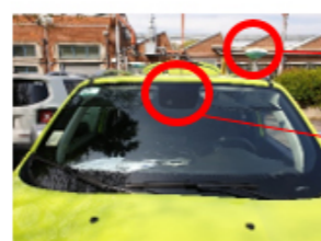
Antenna for DGPS
