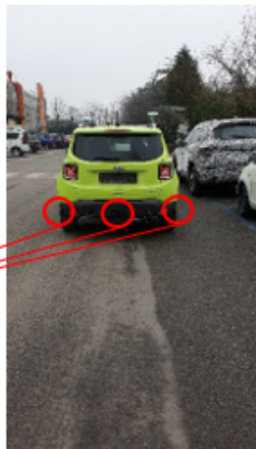
Three rear Laser-scanner sensor
