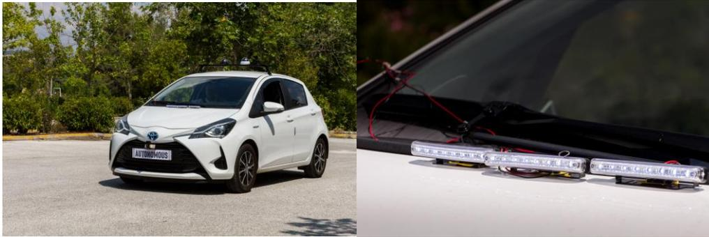
Figure 11: “AV” used in the ICCS study and LED stripe used as eHMI in the condition “AV with eHMI”
