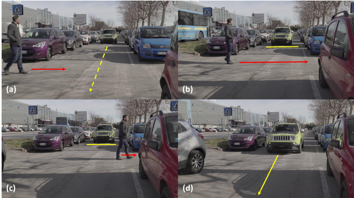
Figure 31: Torino snapshot - Representation of a pedestrian scenario. (a) Potential conflict between pedestrian (red) and AV (dashed yellow) trajectories. (b) AV detects the scenario and decides to stop (yellow stopline). (c) Pedestrian continues his route (HMI green led indication is on). (d) Route is no longer blocked. The AV is safe to continue. HMI led is off.
