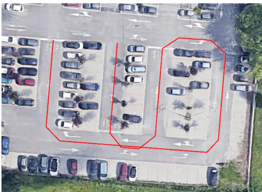
Figure 23: parking scenario for the validation of the Trajectory Planning module, as implemented on the CRF car. The area is the CRF employees parking. The reference trajectory to follow is coloured in RED.
