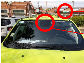
Antenna for DGPS
