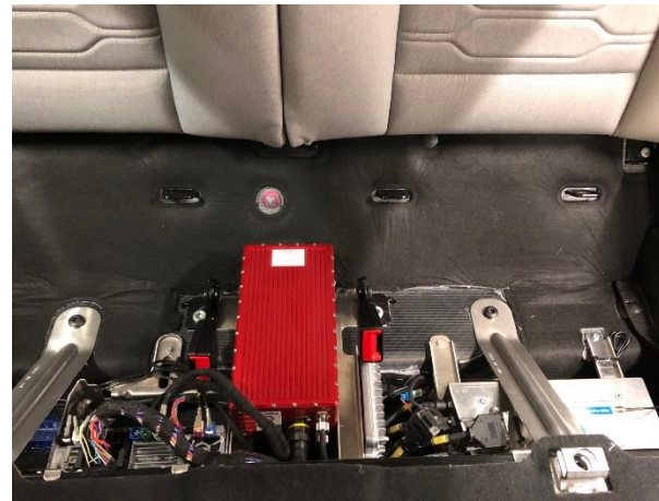
Under back seat (DGPS System)
