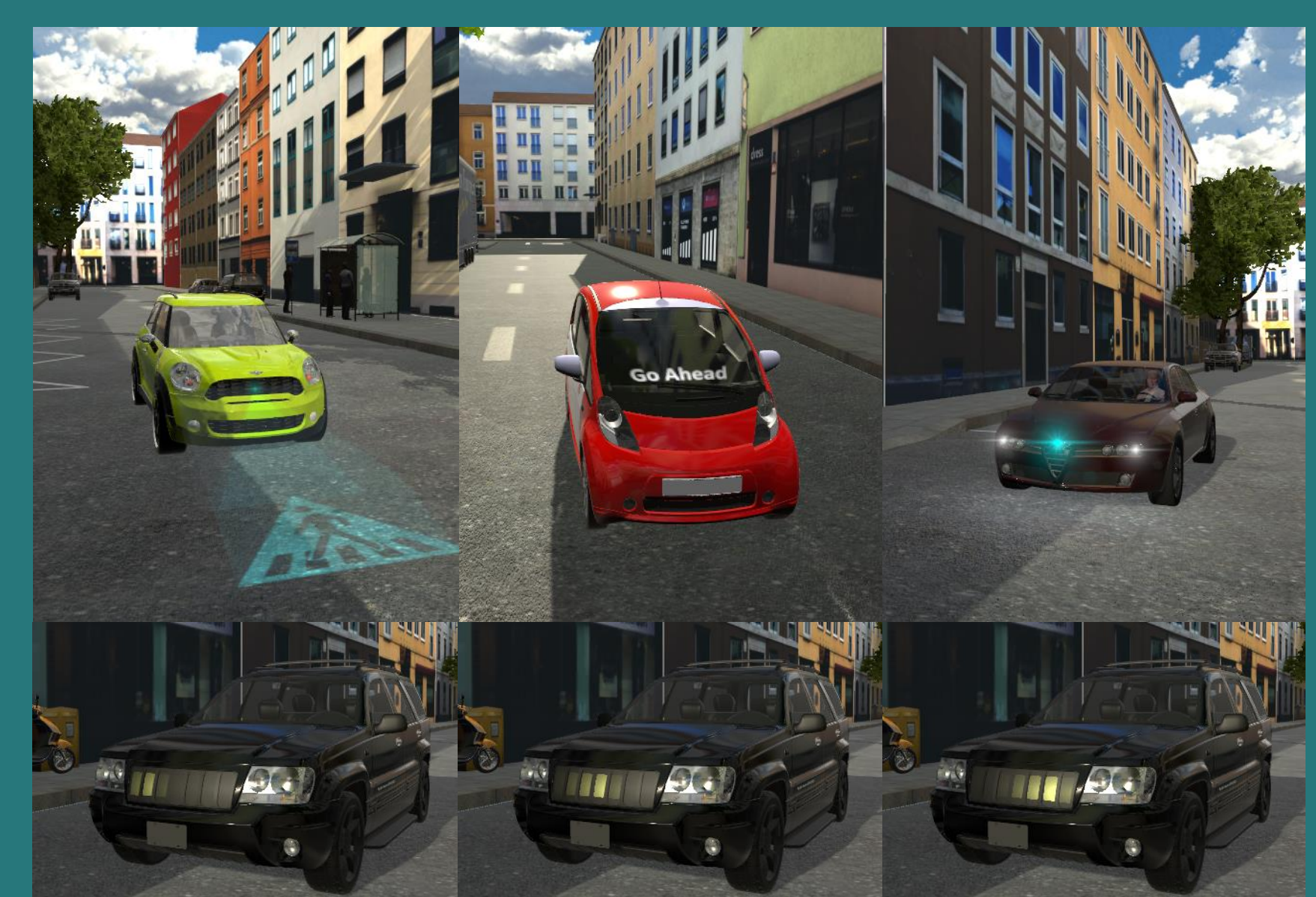
Fig. 3: Pictures from the Pedestrian Simulator at the Technical University of Munich. Potential future communication strategies indicate intentions using different technologies. External Human Machine Interfaces can replace the driver in higher automation levels and extend communication ranges.
