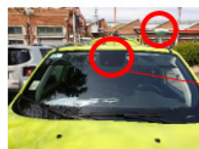
Antenna for DGPS
