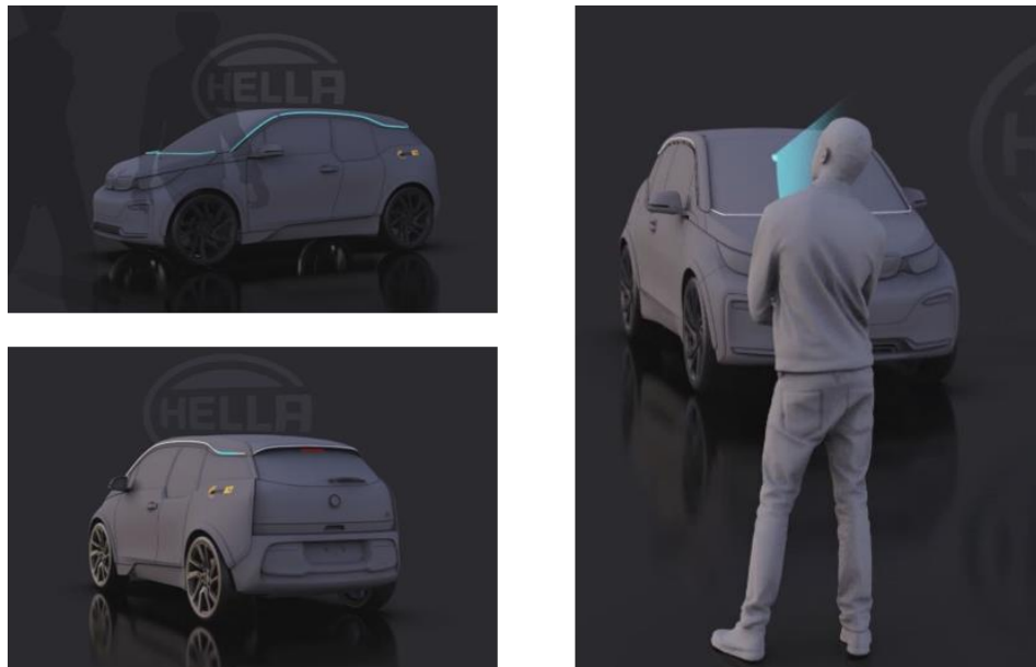
Figure 3: Type, mounting position and light colour of selected eHMI technologies for the BMW i3s – Light Band (left) and Directed Signal Lamp (right).
