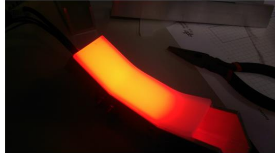
Figure 13: Sketch of the LED stripe (left), bended diffuser for side elements (right).
