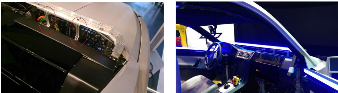
Figure 14: Integration of the 360° Light Band in driving simulator vehicle.
